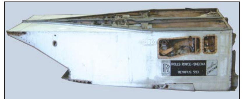
ROLLS ROYCE SNECMA OLYMPUS 593 TWIN AIR INTAKE UNIT
