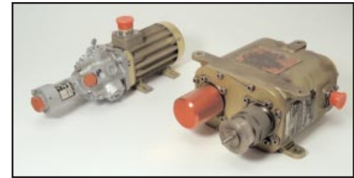
ENGINE REHEAT TRANSFORMER & HISPANO-SUIZA ELECTRIC PUMP
