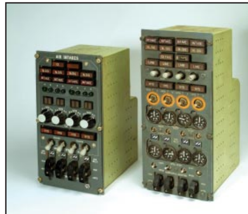
AIR INTAKE CONTROL PANELS
