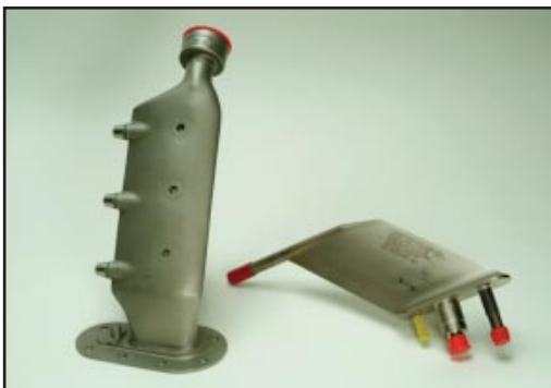
PITOT HEAD & AIR COOLING DUCT
